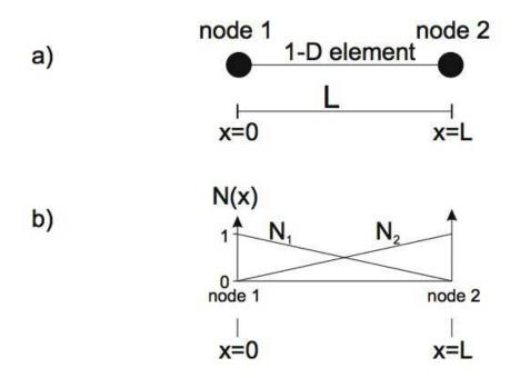
Figure 2: (a) a 2-node, one dimensional finite element with (b) linear shape functions
