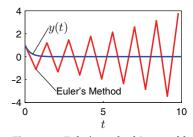
**Figure 8.1** Euler's method is unstable for  $\tau > 2/\gamma$ . ( $\tau = 2.1/\gamma$  in this case.)
