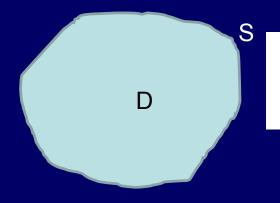
Dirichlet, b. condition: u(x,y=S)=f1
